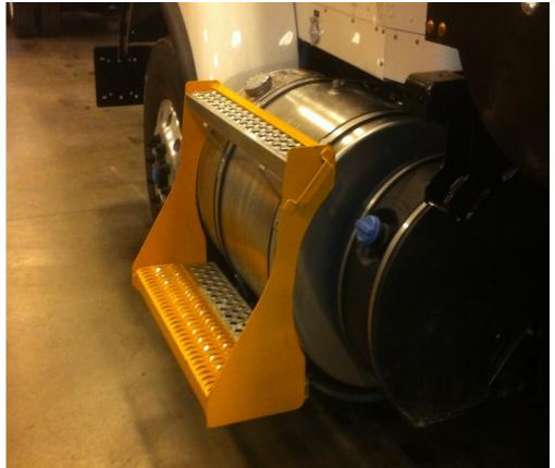
The steps on the driver's side of a truck are not off set, making it difficult to find lower step. By attaching the temporary step, a fall hazard was eliminated
