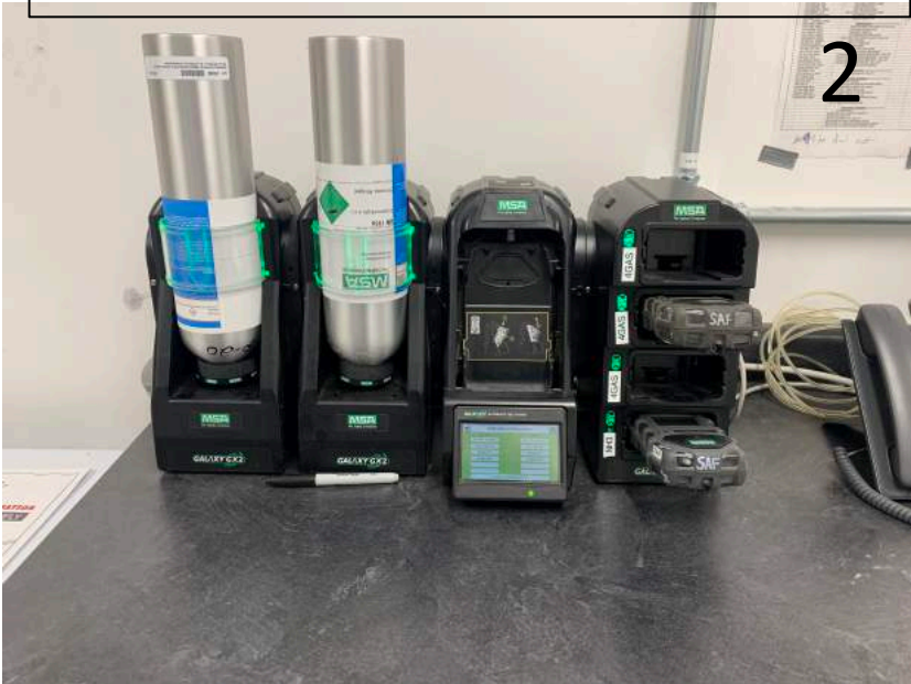
2. MSA Galaxy GX2 Altair 5X Automated Gas Detector Test System
