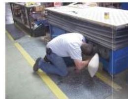
Cleaning of Downdraft Dust Collection systems had been done from below the table surface. Required awkward position and potential breathing in of dust.
