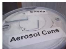
Self-closing door keeps flammable vapors in drum
