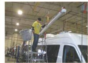
New Method – Hoist installed to assist awning handling. Now requires only one person. Less stress to back and shoulders. Much easier to guide and install.
