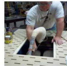
Access from top of table and special vacuum attachment allows easier cleaning.
