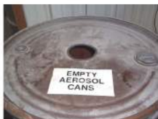
Opening in top of drum potentially allowed flammable vapors to escape
